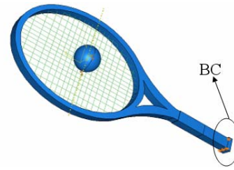
Fig. 2. Boundary condition for string tension analysis.
